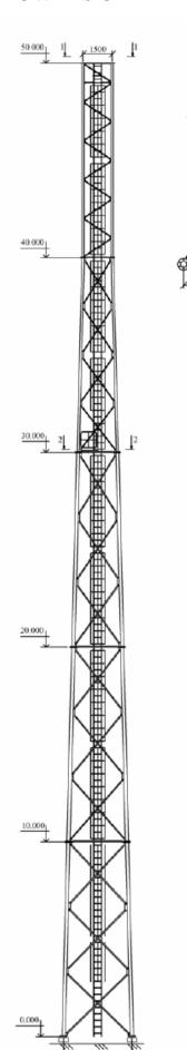
The given series of towers (MT) is designed in accordance with the criteria of a construction optimum cost, technology capabilities during production, unification and easiness at assembly and further technical maintenance. In addition to the said, a small size of basement to the tower allows installing it in small sites.
