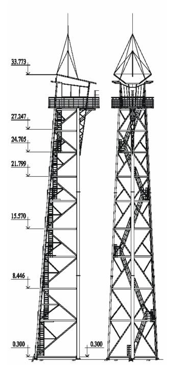
Observation towers (NT) were developed according to the architecture design of the "Arhitektonika" company and were installed within the project framework for reconstruction of the eastern border of the Republic of Latvia.
