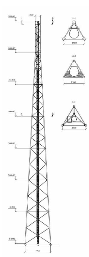
The given series of towers (ST) is suggested to be used in cases when there is a need to install the technological equipment on altitudes ranging from 50.0 to 90.0 metres. At development of the series a requirement to increase the valuable wind loads without deterioration of the required strength features of towers. The main elements and units are designed basing on unification, easiness at assembly and further technical maintenance.
